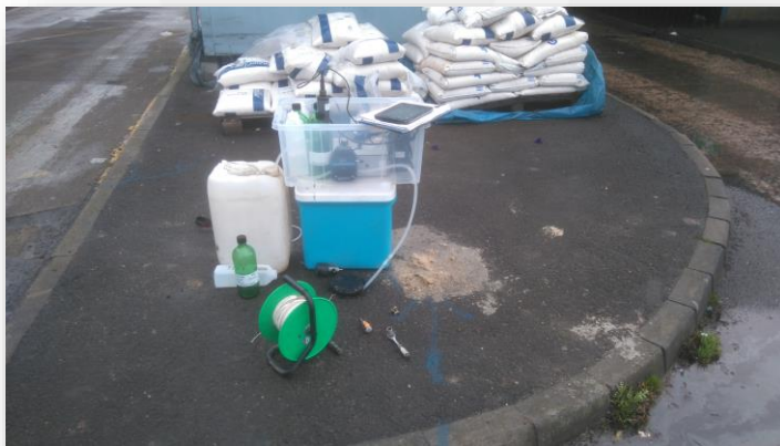
Low flow sampling equipment in operation at standpipe location
