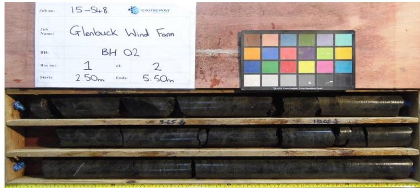
Metric T2-101 core barrel produced excellent core recovery for the Basalt bedrock in 84mm diameter.
