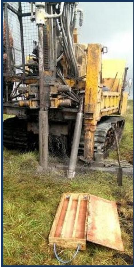
A rotary drilling rig (Beretta T41) mounted on wide tracked low ground bearing carrier.
